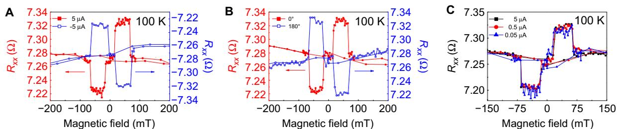
**Fig. 4. Current-dependent transport measurements on FPC3 at 100 K. (A)**  $R_{xx}$ (B) with different current directions. **(B)**  $R_{xx}$  measured when the top FGT layer faces upward ( $0^\circ$ ) and downward ( $180^\circ$ ). **(C)**  $R_{xx}$ (B) with different magnitudes of current.
