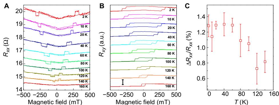
**Fig. 2. Temperature-dependent transport measurement for sample FPC1.** (A)  $R_{xx}$  curves in an FGT/graphite/FGT device at different temperatures. (B) Corresponding  $R_{xy}(B)$  curves at different temperatures. Scale bar,  $3 \Omega$ . (C) Temperature dependence of  $\Delta R_{xx}/R_{xx}$  values. The error bars are defined by the noise level. a.u., arbitrary units.
