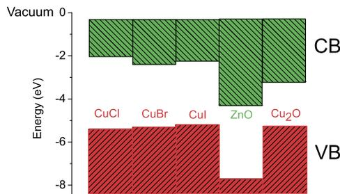
**Fig. 4.** The band offsets among CuCl, CuBr, CuI, ZnO and Cu<sub>2</sub>O. The vacuum level is set to 0 eV. Here the experimental band gap of CuCl (3.39 eV, see Ref. [22]), CuBr (2.91 eV see Ref. [12]), CuI (2.95 eV see Ref. [12]), ZnO (3.4 eV see Ref. [51]) and Cu<sub>2</sub>O (2.1 eV see Ref. [52]) are adopted. The ionization potentials of CuI (5.2 eV), ZnO (7.7 eV), and Cu<sub>2</sub>O (5.3 eV), are taken from the literature see Refs. [50–52].
