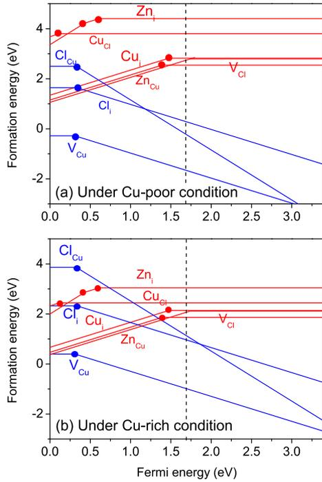
**Fig. 2.** Formation energy of intrinsic defects and extrinsic Zn-related defects in  $\gamma$ -CuCl under two different chemical potential conditions, *i.e.* Cu-poor (a) and Cu-rich (b). Red and blue lines represent the donor and acceptor defects, respectively. Here the experimental band gap [22] of  $\gamma$ -CuCl  $E_g = 3.39$  eV is adopted. The vertical dashed line represents our calculated band gap.
