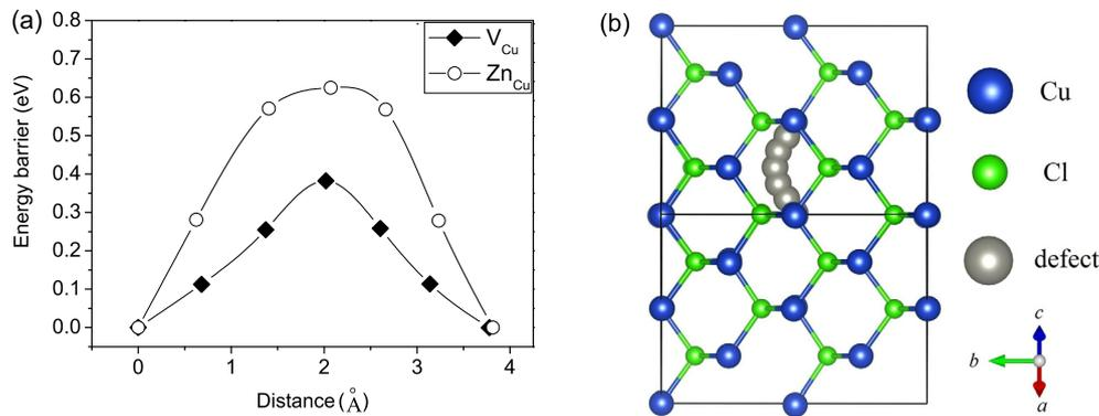
**Fig. 3.** The calculated diffusion barriers (a) of  $V_{Cu}$  and  $Zn_{Cu}$  from a centered tetrahedron site to a nearby centered site in  $\gamma$ -CuCl and the diffusion path (b) in our used supercell.
