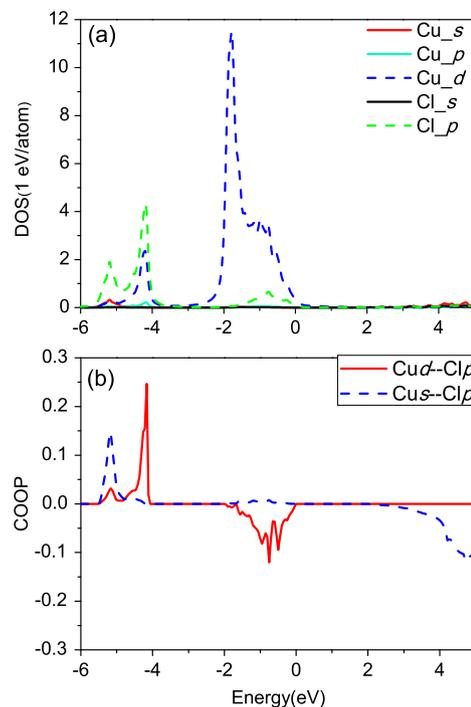
Fig. 1. The partial density of states (a) and the COOP (b) in  $\gamma$ -CuCl. The valence band maximum is set to zero.
