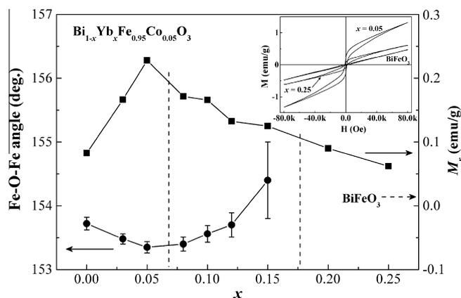
**Fig. 4.** The remanent magnetization  $M_r$  of BYFCO powders and the Fe–O–Fe angle of the *R3c* lattices as the function of the doping concentration  $x$ . The inset shows the hysteresis loops of BFO and BYFCO with  $x = 0.05$  and  $x = 0.25$ .
