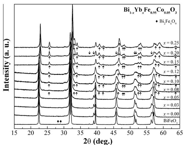
Fig. 1. XRD patterns of BFO and BYFCO powders. The upward arrows indicate the new peaks and the downward arrows indicate the vanishing peaks as  $x$  increases.
