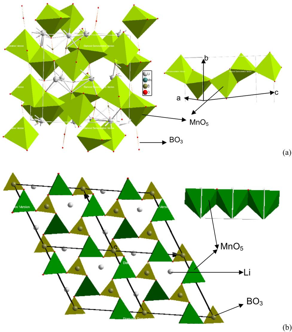
**Fig. 1.** The three-dimensional framework of LiMnBO<sub>3</sub>: (a) monoclinic structure; and (b) hexagonal structure.
