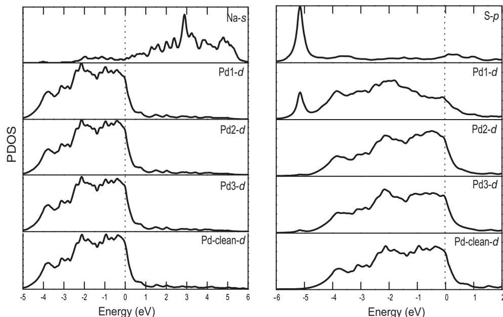
FIG. 5.  $d$ -PDOS of the Pd atoms in clean Pd: Na/Pd (a) and S/Pd (b) before CO adsorption. The numbers “1,” “2,” and “3” with “Pd” stand for the first, second, and third nearest neighbor relative to the adatoms (S and Na), respectively. The Fermi level ( $E_F$ ) is set to zero.
