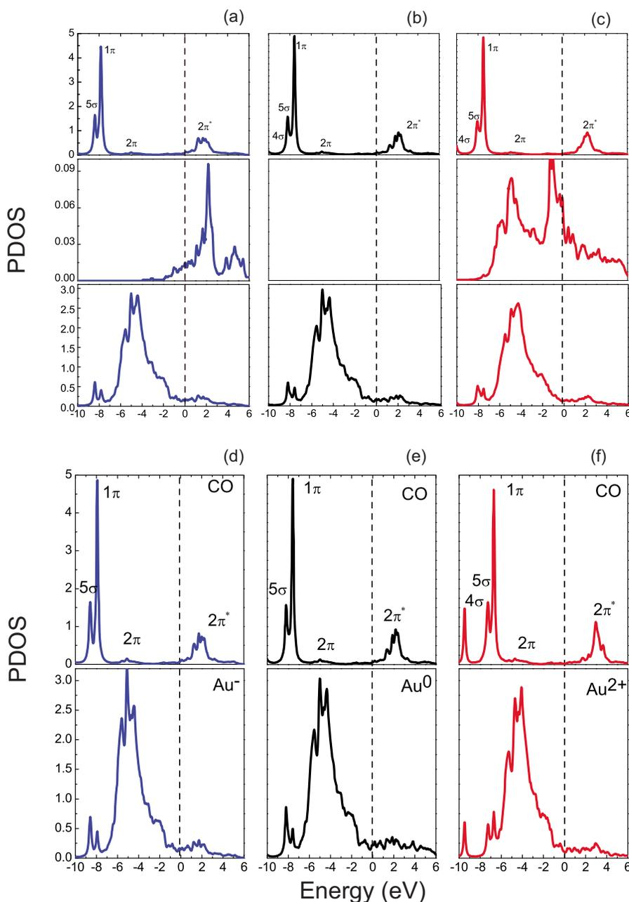
FIG. 4. PDOS of CO adsorbed on Na/Au (a), clean Au (b), S/Au (c), and  $\text{Au}^\delta$  surfaces ( $\delta=1-, 1+, \text{ and } 2+$ ) [(d) and (e)]. The Au atoms employed here are those that bond to CO. The Fermi level ( $E_F$ ) is set to zero.
