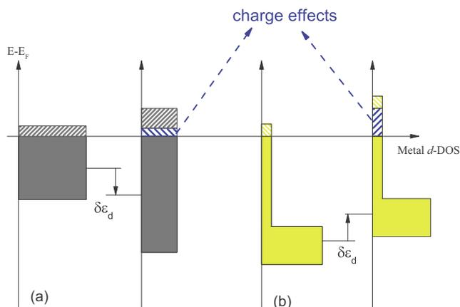
FIG. 7. Sketch of metal  $d$  band changes after S, Cl, and O adsorption on TM (a) and on Au or Ag (b). In Au and Ag, the center of  $d$  band is shifted up since the charge effects dominate over the poisoning effects, while the poisoning effects prevail on TM. The blue areas indicate the induced charge effects.
