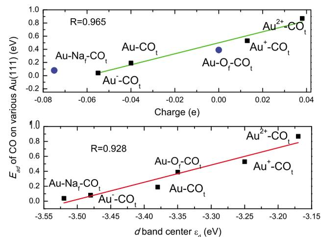
FIG. 3. CO adsorption energies,  $E_{ad}$  (eV), vs net charge (upper panel) and  $d$  band center (lower panel) of Au atoms ready to bond with CO. Since the effects of O and Na on CO adsorption are the most remarkable, as seen in Table I, only O and Na preadsorbed Au are depicted in the upper panel and emphasized through blue solid circles.
