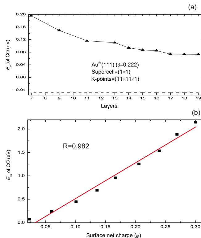
FIG. 8. (a) Convergence test of CO adsorption on the Au surface with a charge of  $+0.222e$ , with respect to the number of layers in the substrate; with dashed line showing the adsorption energy of CO on neutral Au(111) with the same coverage. (b) CO adsorption energy as a function of the surface net charge with a 17-layer slab model.
