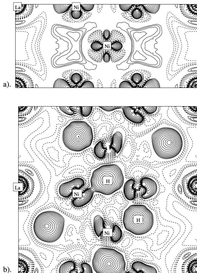
FIG. 3. The bonding charge density plot for optimized (a).  $\text{LaNi}_5$  and (b).  $\text{La}_2\text{Ni}_{10}\text{H}_{14}$  along  $(2\bar{1}10)$  plane within GGA. Contours start from  $10^{-3} e/\text{a.u.}^3$  and increase successively by a factor of  $\sqrt{2}$ . The solid and dashed lines denote the accumulation and depletion of charge density in comparison with the superposition of atomic density.
