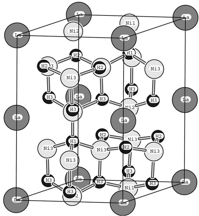
FIG. 1. The ball-stick model for the structure of  $\text{La}_2\text{Ni}_{10}\text{H}_{14}$  labeled with the different atom types.
